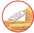
Fusible links hold doors wide open and melts at 74°C for automatic closure (on self-close models).
